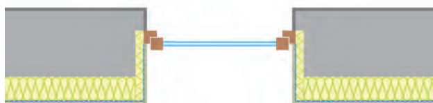
Solution 3: internal insulation
