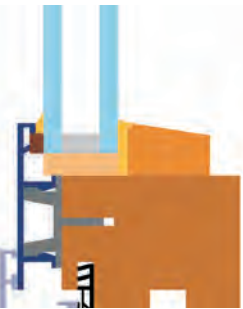
↑ Illustration 212: Frame in wood and aluminium
