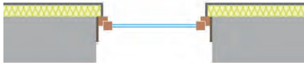
Solution 1 : external insulation
