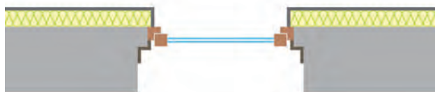
Solution 2: external insulation
