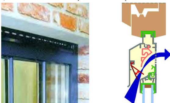
↑ Illustrations 92 and 93: Grilles for air intake in new frames
