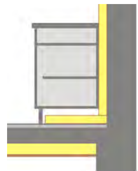
↑ Illustration 153 : Insulation by inside (floor and wall)
