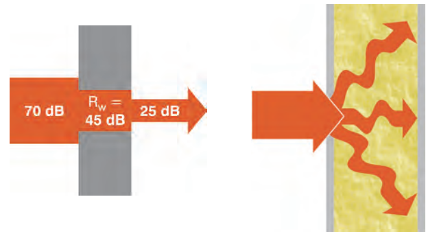
↑ Illustration 103 : Noise attenuation thanks to walls
