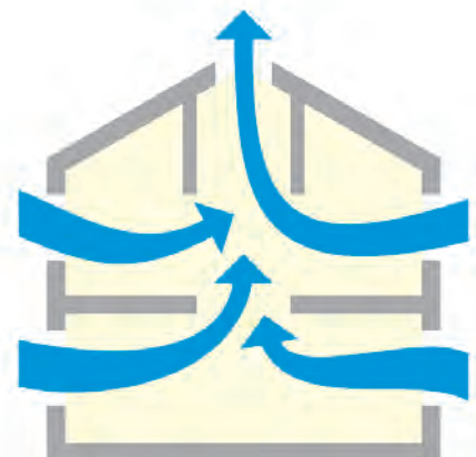
↑ Illustration 197: Type of natural ventilation - Air flows
