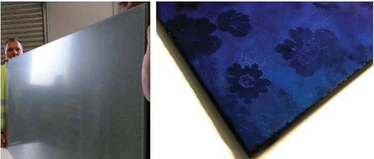
Figure 17: Different surfaces: smooth, flat and uncoated (left), structured with spectrally selective coating for higher thermal yields (right). © Fraunhofer ISE.
