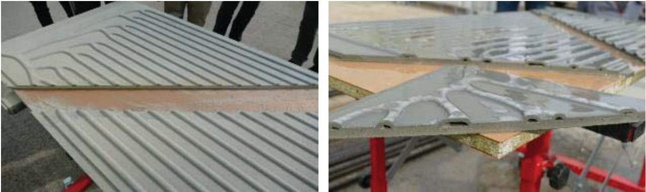
Figure 16: Cuts of TABSOLAR element showing fluid channels on the back side. © Fraunhofer ISE.
