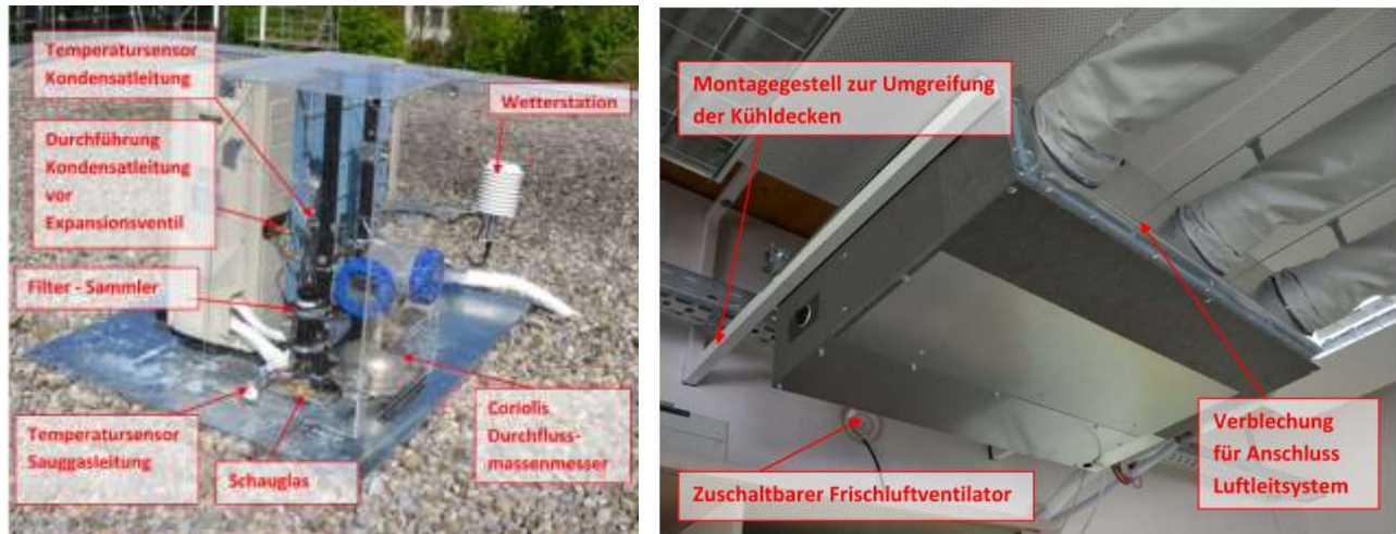
Figure 11: Installation of brand supplier Mono-split-unit at ZAE Bayern [EvaSolK 2013]
