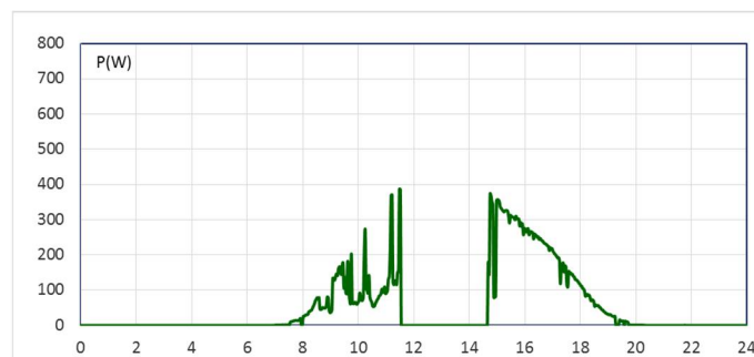
Figure 8 Field measurements of the electrical energy consumed in the electrical heater by joule effect
