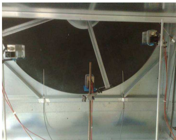
Figure 25: Psychrometers and temperature sensors distribution at the outlet of the desiccant wheel
