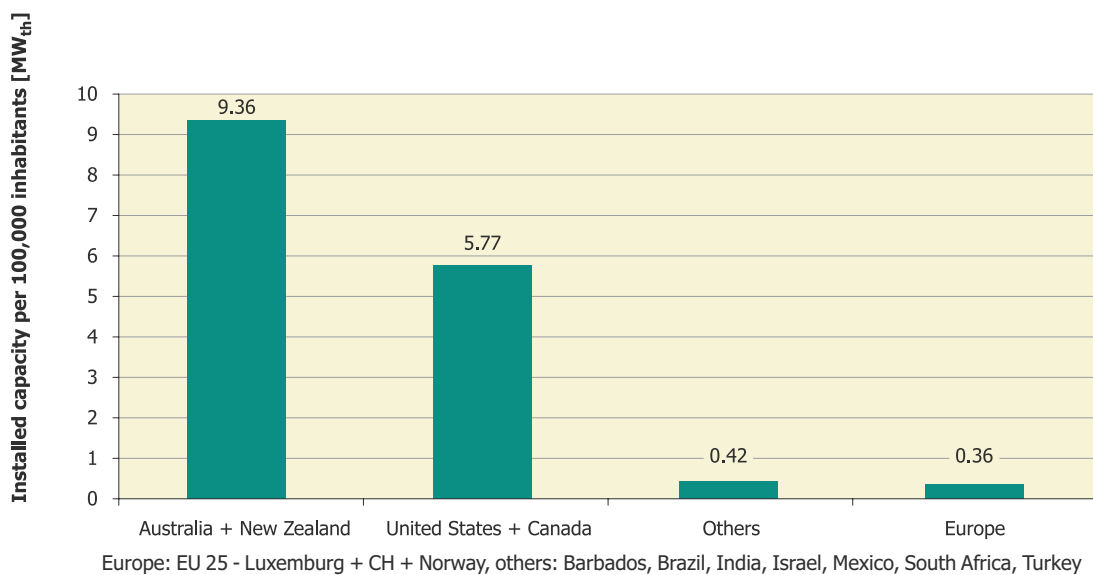
Figure 12: Cumulative installed capacity of unglazed collectors in operation by economic region at the end of 2004 per 100,000 inhabitants
