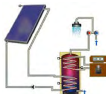
Figure 34: Hydraulic scheme of the DHW reference system
