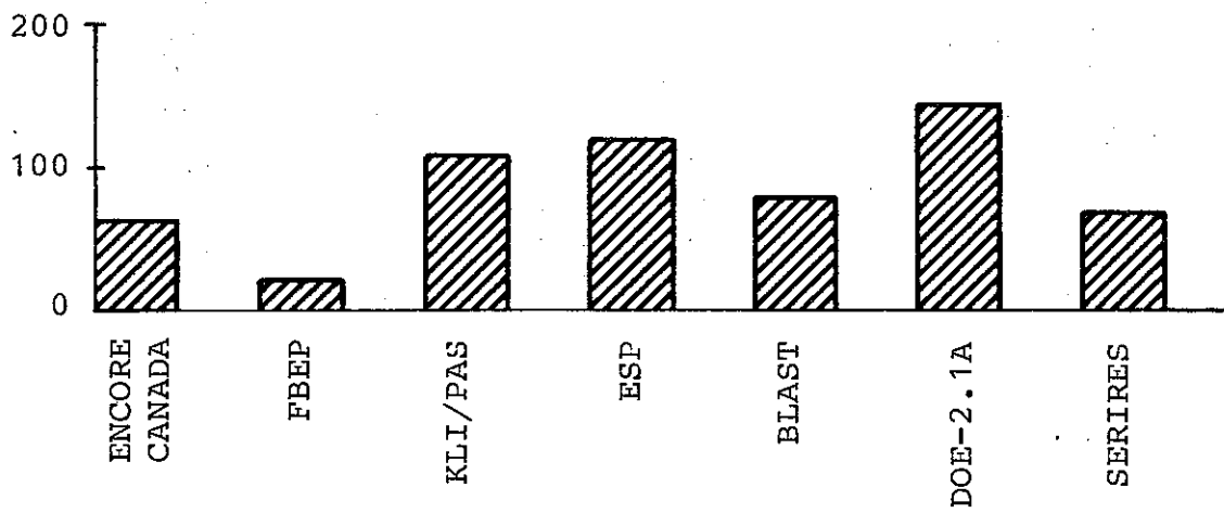
Fig. 5.35 Comparison of cooling requirements for Copenhagen.
