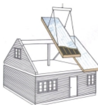
(d) collector as factory prepared roof unit
