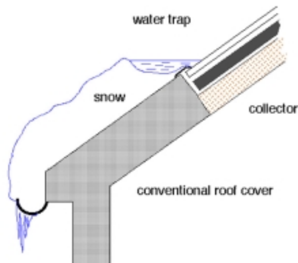
Fig. 3 Snow accumulation on a partly covered collector roof
