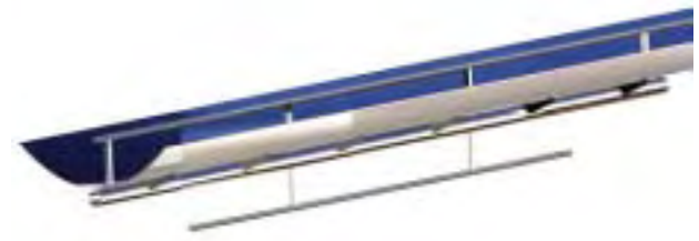
CAD model of the PolyTrough 1200
