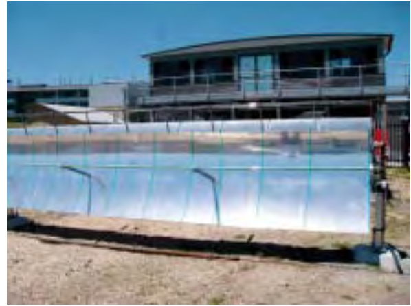
Reflectors adhered to the mirror for photogrammetry tests
