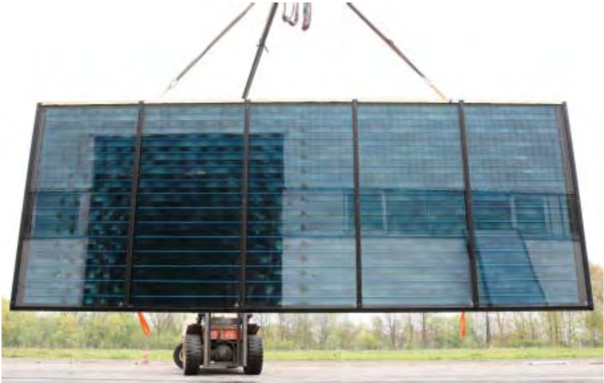
10.5 m 2 collector ready for transport on truck or shipping in a standard container
