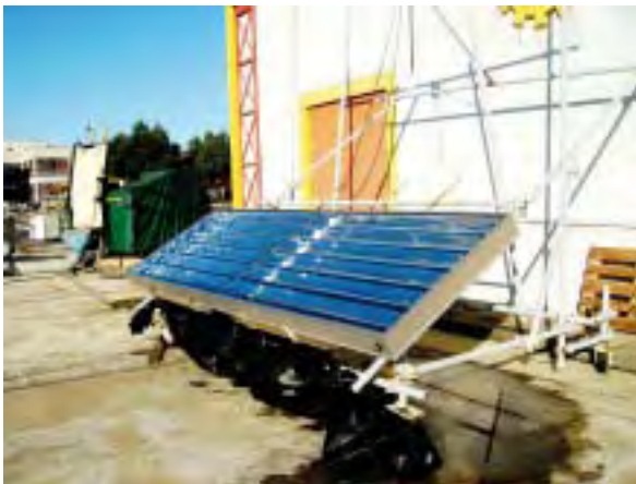
Prototype MAXI collector being tested at INETI
